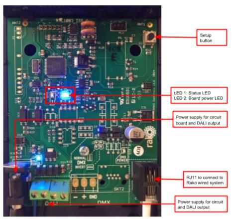
The WSR-DALI must be connected to the Rako wired system by the RJ11 port either plugged directly to RAKLink or RAKStar or punched down to the CAT5 cable via a WP-CONC. The WSR-DALI requires 18V DC, a suitable power supply attached to a 13A plug is provided with the product. When successful powered up LED 2: the "Power LED" will illuminate.
