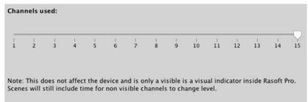
Slide the "channels used" slider to match the number of Channels required by the WSR-DALI and the remaining channels are freed up to be used by other devices.
